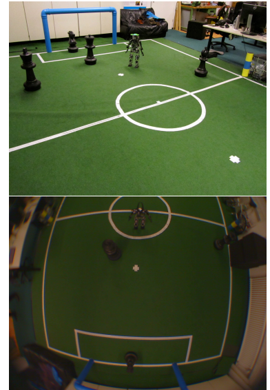
Figure 10.1: The evaluation setup: the robot is wearing the special markers and is tracked by the overhead camera system.
